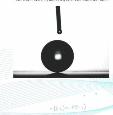
(3) Unique interface tension measuring system of liquid-gas / liquid-liquid with Young-Laplace equation fitting method based on Bashford-Adams table, ADSA® (Runge-Kutta arithmetic and Realdrop® method) and capillary pressure method. It can be used for surface tension measurement of medium-high viscosity sample, dynamic surface / interface tension measurement of surfactant, and oscillating drop measurement.
